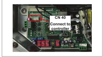
Figure 26 Location of CN40 Port for 2x2 (9-18K) Units
