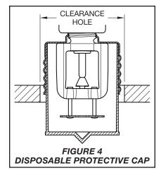
Do not attempt to compensate for insufficient adjustment in the sprinkler by under- or over-tightening the sprinkler/support cup assembly. Re-adjust the position of the sprinkler fitting to suit.
