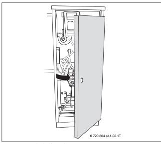
Fig. 2 Open boiler front door
