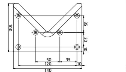
Screws / vis 15x D 5 mm - L 20 mm
