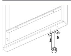
For ladder depth: 320 mm (12 5/8") Height: 100 mm (4")
