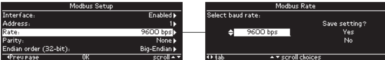
Fig. 43. Modbus baud rate setup
