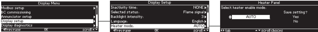
Fig. 62. Heater mode setup
