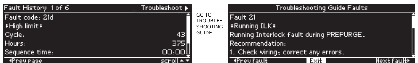
Fig. 21. Troubleshooting guide from fault history record
