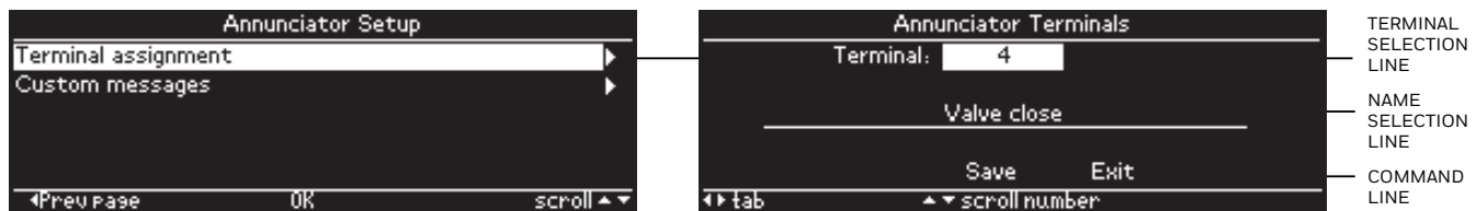
Fig. 47. Annunciator terminal assignment setup
