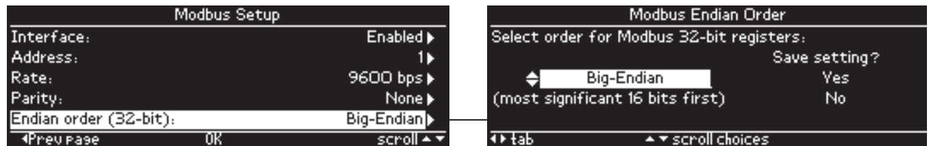
Fig. 45. Modbus Endian order setup
