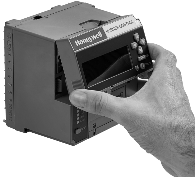
Fig. 2. Keyboard Display Module mounting.
