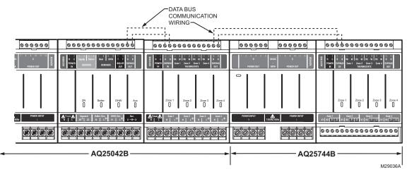
Fig. 7. Wiring for communication bus.
