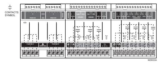
Fig. 2. Internal wiring for AQ2000 Series components line voltage relays.
