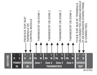
Fig. 8. Connecting thermostats.
