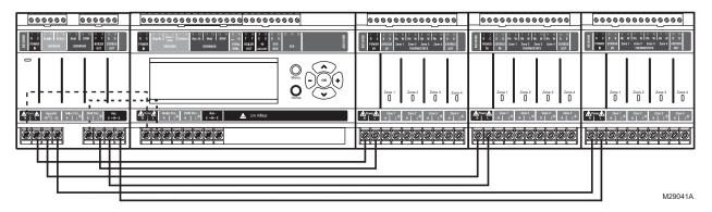
Fig. 18. Connections for multiple Zoning Panels - parallel wiring.
