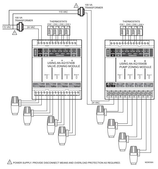
Fig. 13. Wiring of additional low voltage VA capacity.
