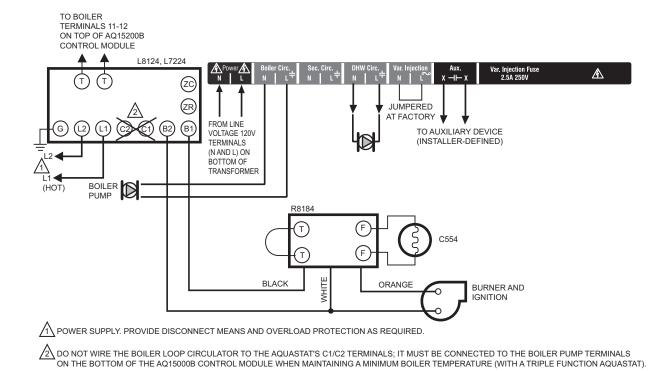
Fig. 14. Line Voltage Connections for AQ250.
