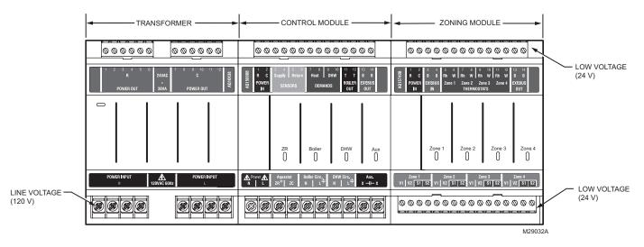
Fig. 1. AQ250 Control Panel layout (AQ25044B shown).
