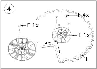
Assemble the Arrestor assembly Drop in (E) nut, then attach the (L) pole bracket to the (I) arrestor
