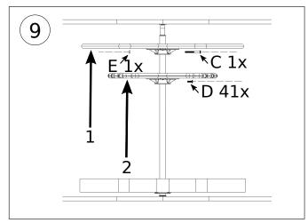
Raise the Top Plate assembly up (1), Install the (E) Nut and (C) Bolt. Raise the Arrestor assembly up (2), Install the (D) Screw and adjust height
