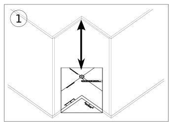
Use the provided template to center the (B) pivot bracket on the top and bottom of the cabinet
