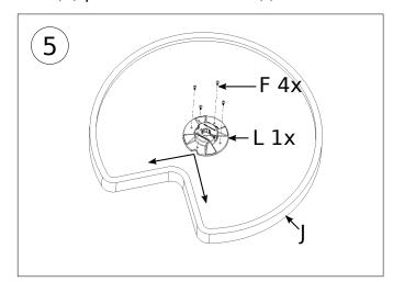
Assemble the Bottom Shelf Attach the (L) pole bracket to the under side of the (J) bottom shelf
