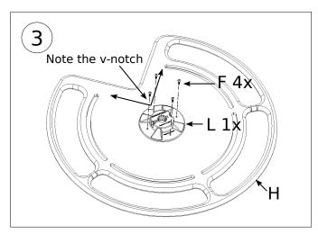
Attach the (L) pole bracket to the (H) top plate
