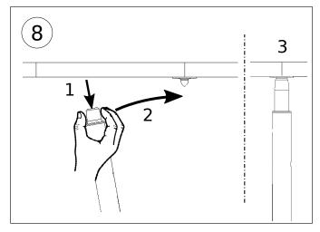
1 Pull down on the top pin, 2 locate the pole above the pin 3 Release the pin to lock into position
