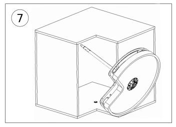
Insert the pole assembly into the cabinet
