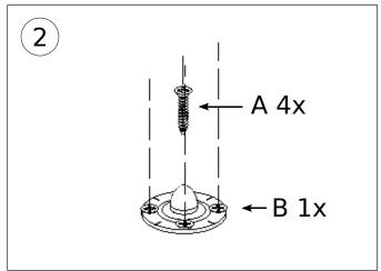
Mount the pivot bracket Top & bottom of the cabinet
