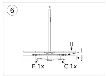
Add the Top Plate, Hand Rail, and Shelf to the (K) Pole, then bolt the bottom shelf using (C) and (E) nut throuh the pole mounting hole. Tighten firmly
